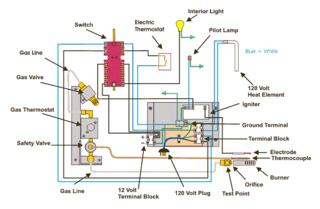
Note: In the graphic above, the switch and electric thermostat are shown for clarity. The switch really lies in front of the gas valve and can't be seen from the rear. The switch is accessed by removing the gas controls in front of it. The electric thermostat is located inside the refrigerator.
